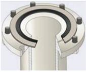
The construction of this gasket is a circular metal winding with an outer centering ring. The sealing element is made of alternating plies of a specified metal and soft sealing material. Standard pipe size gaskets are made to ASME B16.20 (see also style 913M). These gaskets are used in a wide variety of applications.
